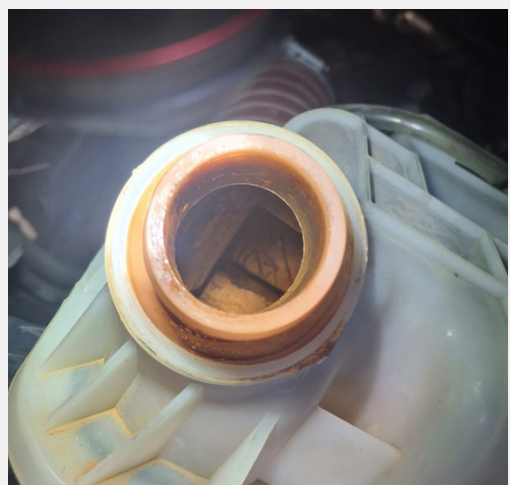
Corrosion in cooling system due to lack of maintenance
