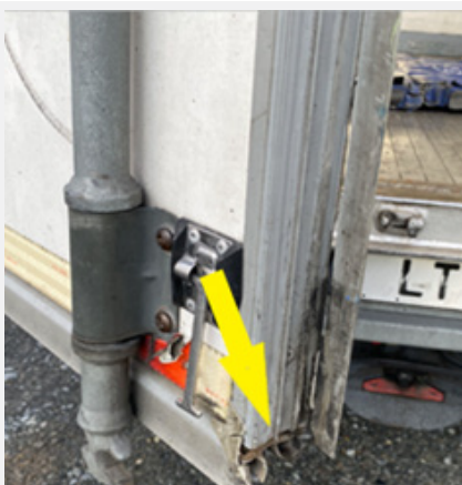
Excessively worn door seals
