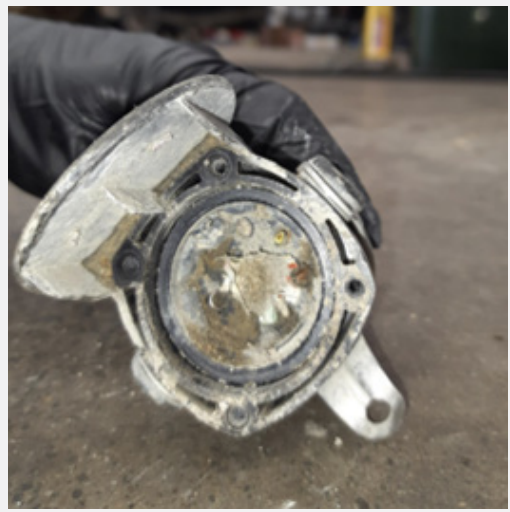
Connections & plugs broken or worn out
