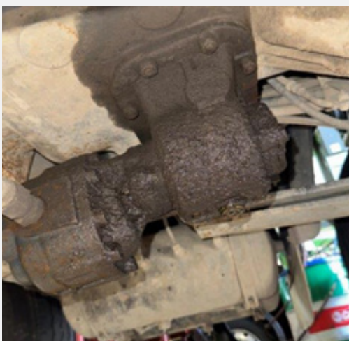
Transmission oil leak requiring repair
