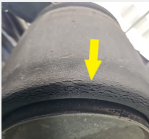
Excessive cracking on air bag
