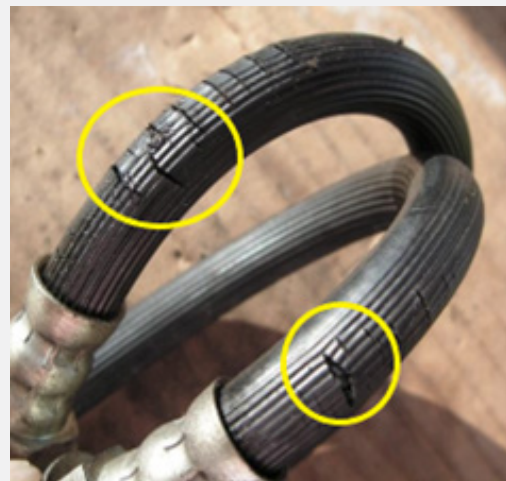
Cracked and perished brake hose
