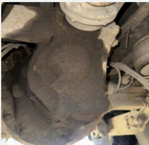
Diff oil leak requiring repair
