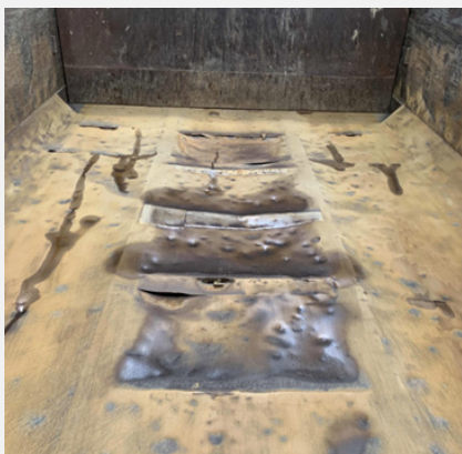
Excessively worn tipper bin
