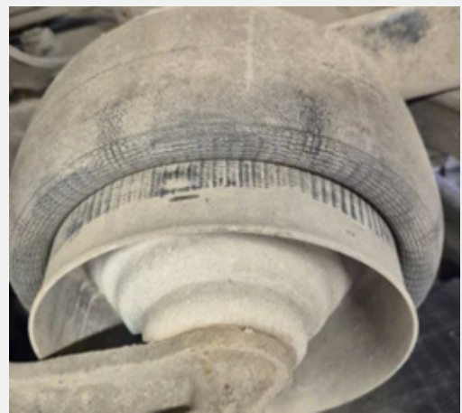
Minor cracking on air bag expected for age
