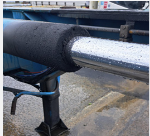
Oil misting from cylinder from normal usage
