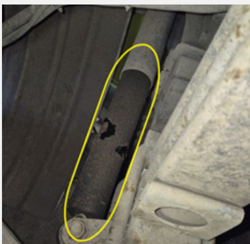
Leaking shock requiring replacement
